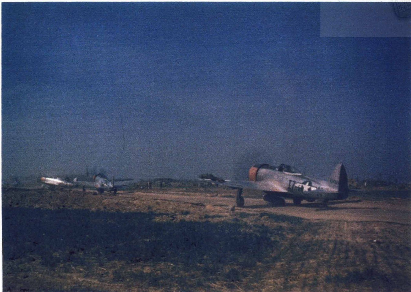
KELZ/DUREN, GERMANY 493rd (I-7) AIRCRAFT READY FOR TAKE OFF, NOTE EXTER- NAL GAS TANK AND MECHANIC ON WING, GUIDING PILOT
